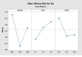
Fig: 1. Main effects plot for Ra
